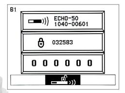
4. 1040-00601 is the transmitter identification number and 032583 is the prompt code in the diagram. Use and to input password in
