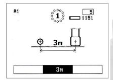
6.Tap two times to start 3m/10/20m calibration and wait for calibration to complete.
